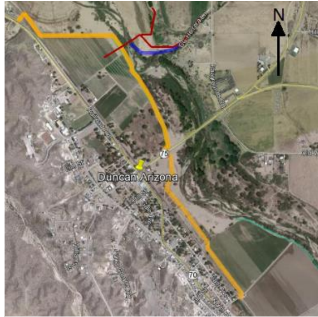
Figure 1.3 - Location of current levee in Duncan. The yellow line running along the west side of the river exhibits the current levee in place [6].
